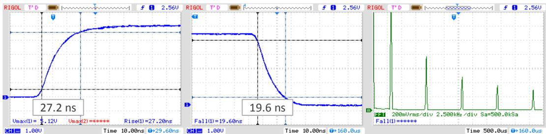
Figure 4.1: PWM signal characteristics at the microcontroller output.
