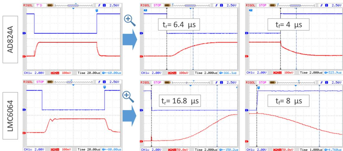
**Figure 4.3:** Evaluation of LMC6064 and AD824A speed. Blue: PWM reference, red: modulated LED current signal. Measured over  $1\Omega$  resistance with inverted analog switching logic using DAC level 4.
